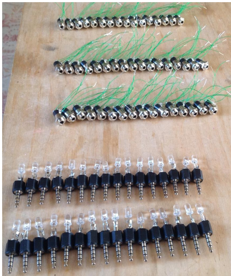
Figure 6: the completed jacks and jack sockets
